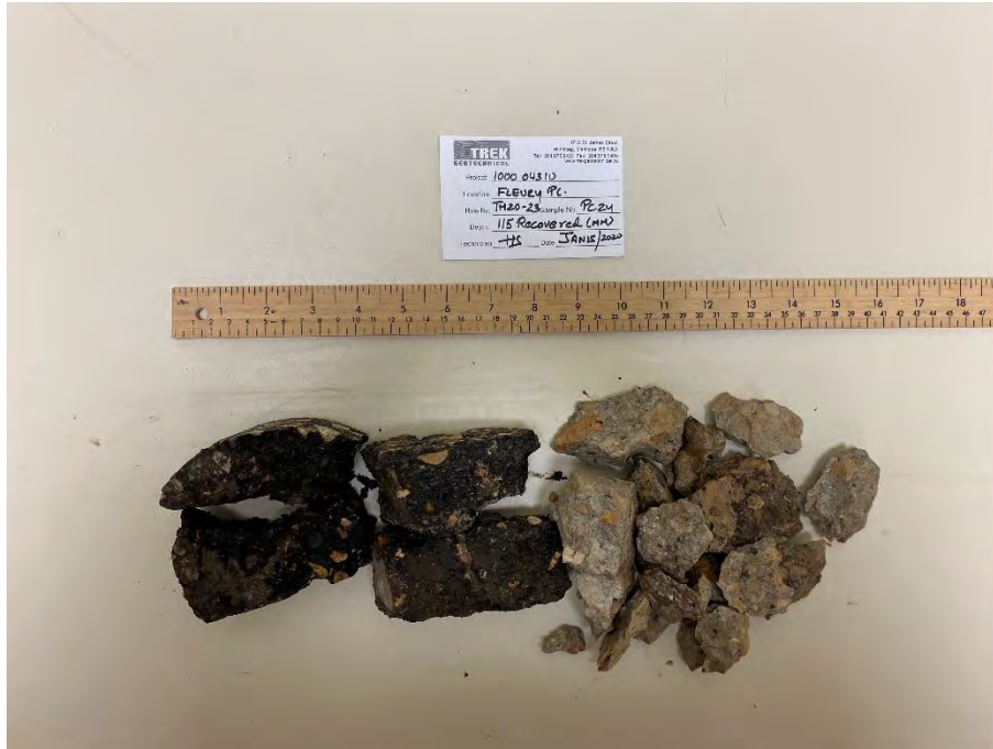
Photo 1: Pavement Core Sample at Test Hole TH20-23
