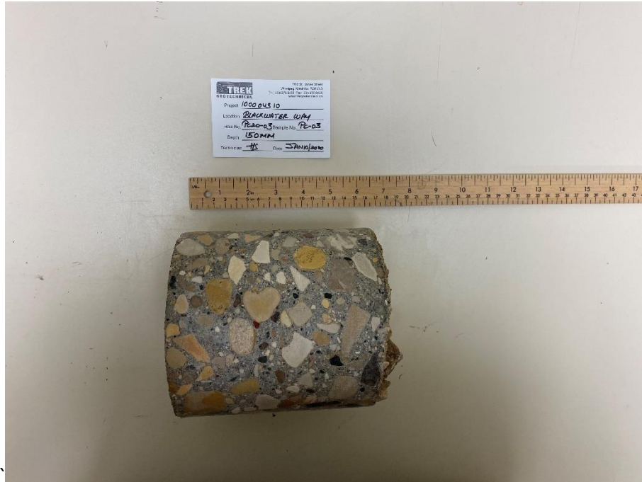
Photo 3: Pavement Core Sample at Test Hole PC20-03
