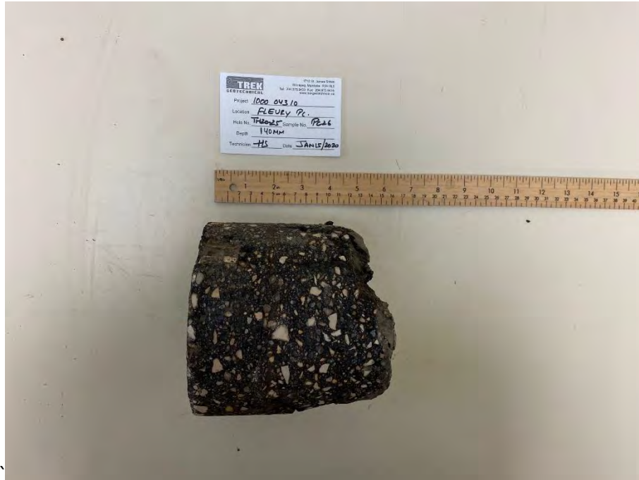
Photo 3: Pavement Core Sample at Test Hole TH20-25
