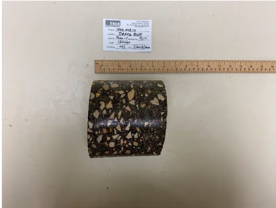
Photo 5: Pavement Core Sample at Test Hole PC20-17
