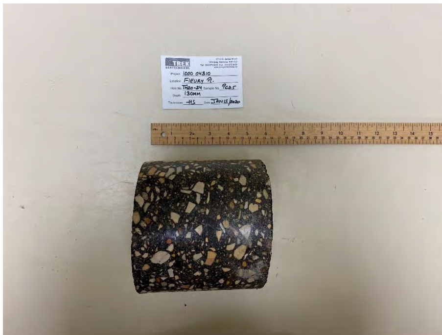
Photo 2: Pavement Core Sample at Test Hole TH20-24
