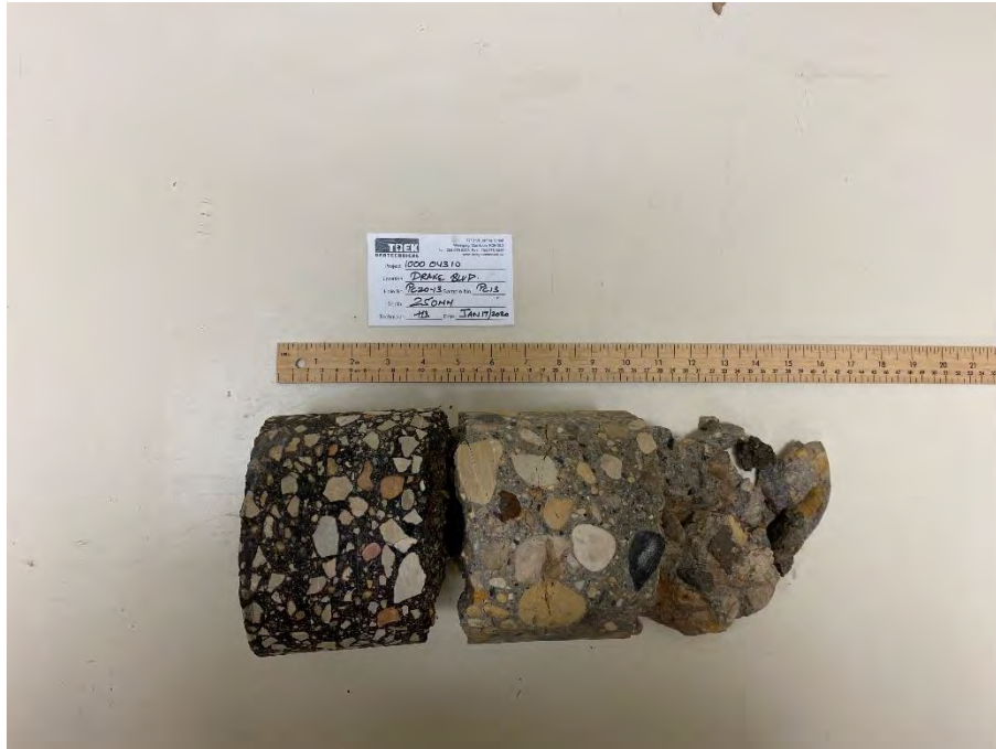
Photo 1: Pavement Core Sample at Test Hole PC20-13
