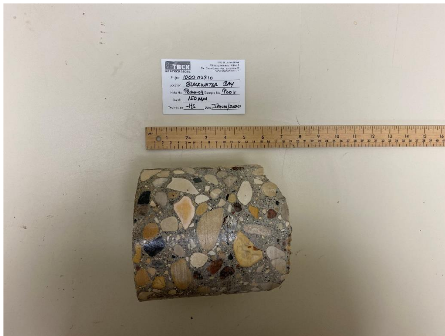
Photo 4: Pavement Core Sample at Test Hole PC20-04
