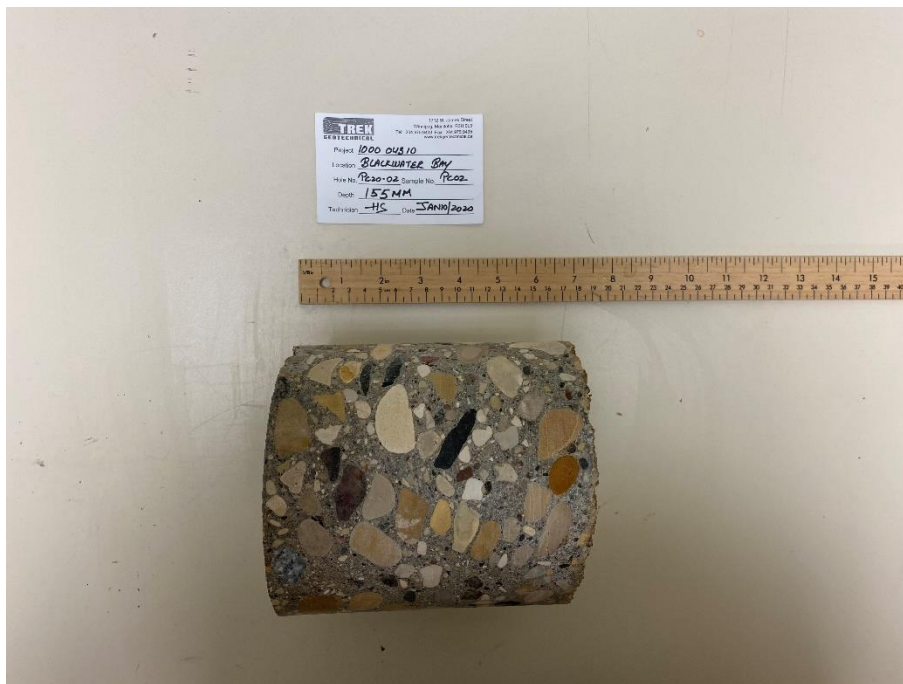
Photo 2: Pavement Core Sample at Test Hole PC20-02
