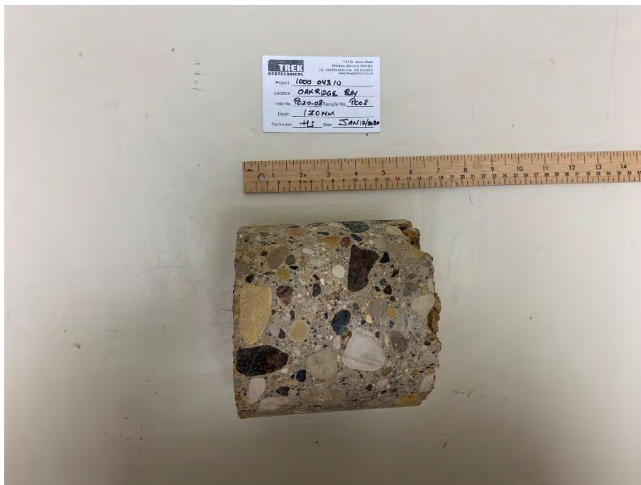
Photo 2: Pavement Core Sample at Test Hole PC20-08
