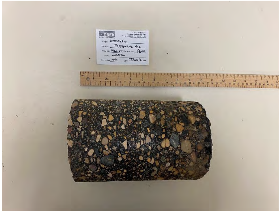
Photo 1: Pavement Core Sample at Test Hole TH20-27
