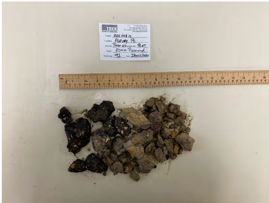
Photo 4: Pavement Core Sample at Test Hole TH20-26
