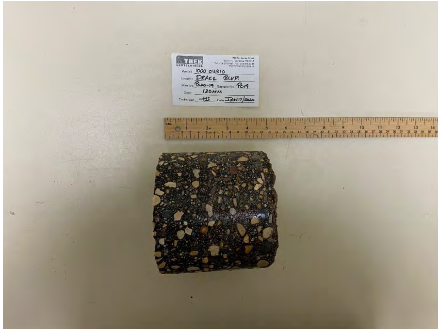
Photo 7: Pavement Core Sample at Test Hole PC20-19
