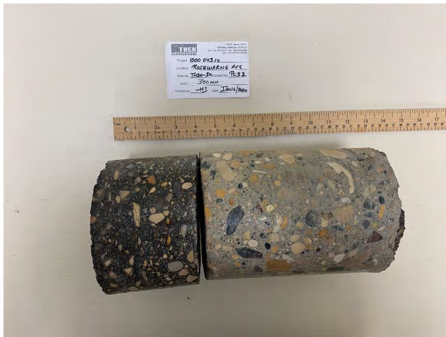
Photo 4: Pavement Core Sample at Test Hole TH20-30
