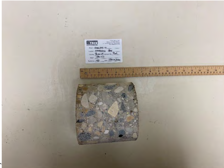
Photo 3: Pavement Core Sample at Test Hole PC20-09
