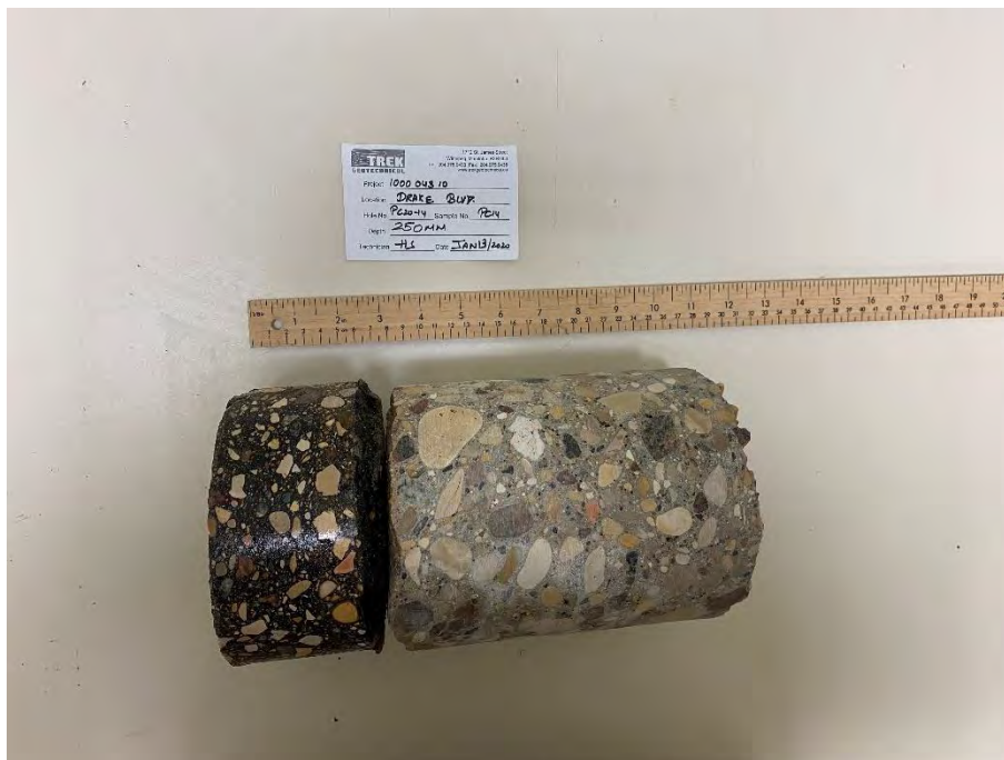
Photo 2: Pavement Core Sample at Test Hole PC20-14
