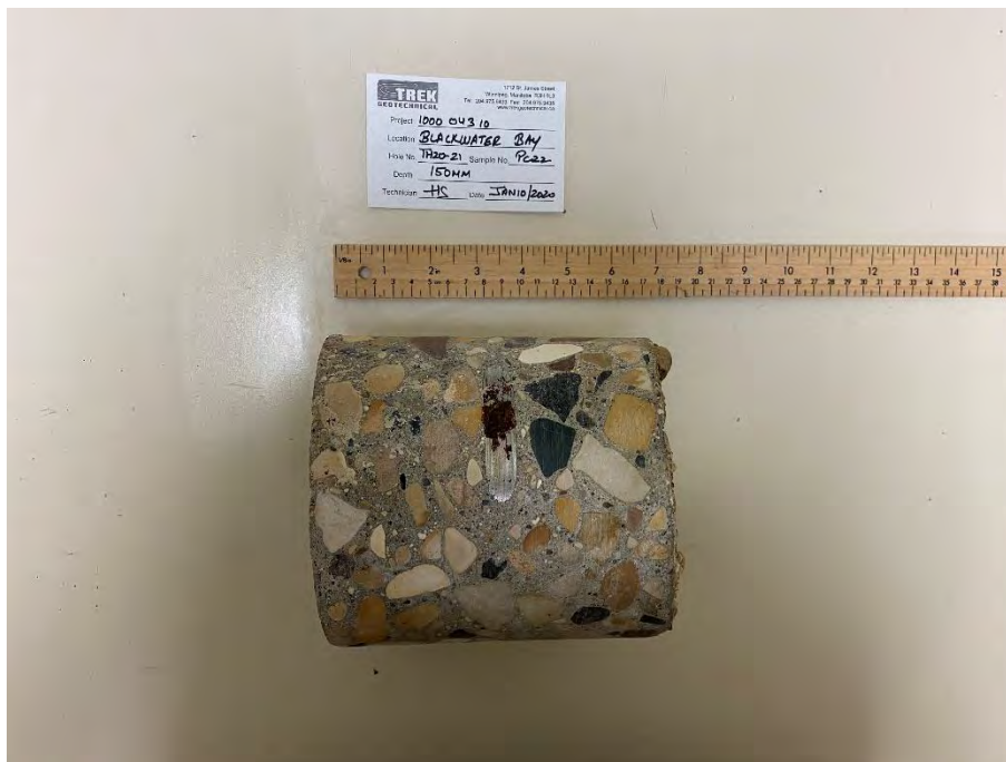
Photo 2: Pavement Core Sample at Test Hole TH20-02
