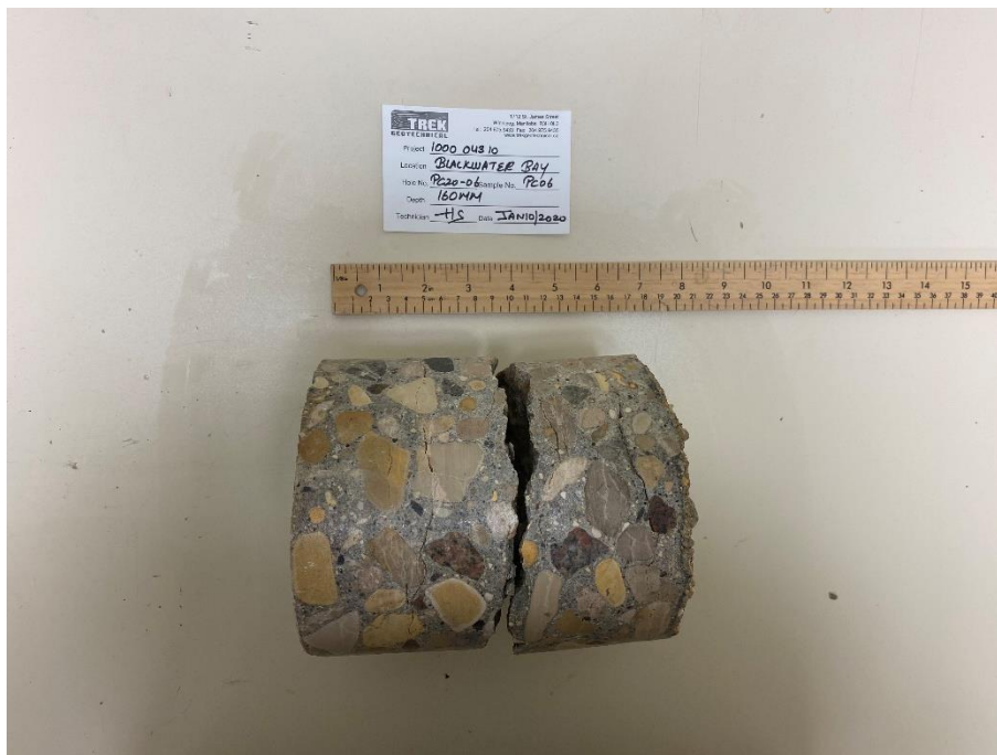
Photo 6: Pavement Core Sample at Test Hole PC20-06
