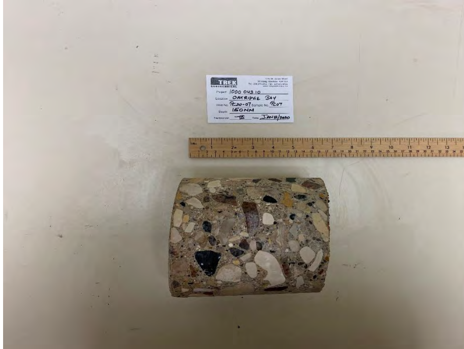
Photo 1: Pavement Core Sample at Test Hole PC20-07
